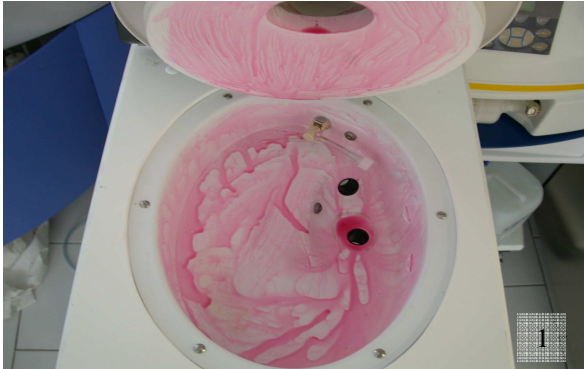
Photos 1 and 2: Controls: Aspect of internal surfaces of the chamber and of external surfaces of the surrogate device after contamination.
