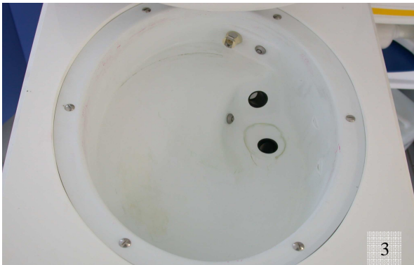
Photos 3 and 4: Assays: Aspect of internal surfaces of the chamber and of external surfaces of the surrogate device after contamination and cleaning by the SL-ENT-APA (SOLUSCOPE SAS) standard cycle (see table I, phases 1 to 4).
